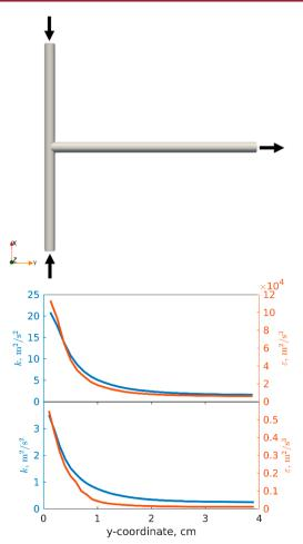
**Figure 4.** Spatial evolution of TDR,  $\varepsilon$ , (red line) and kinetic energy, k, (blue line) over the mixing channel length. Case study operative conditions:  $T_{2mm}$ -mixer, 12.3 m/s velocity in the mixing channel namely flow rate of cases #1–5 (top).  $T_{2mm}$ -mixer, 4.1 m/s velocity in the mixing channel, namely the flow rate of case #7 (bottom).
