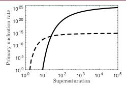
Figure 11. Homogeneous nucleation rate (solid line) compared with the heterogeneous one (dashed line) using the inferred primary nucleation parameters.
