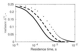
**Figure 5.** Variance evolution obtained using the TDR and kinetic energy from CFD simulations as a function of the residence time (s) for three flow rates (cases #5–7). The solid line refers to case #5, the dashed line refers to case #6, and the dotted line refers to case #7.
