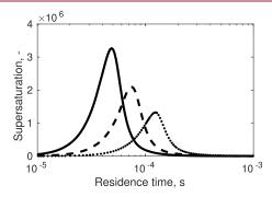
**Figure 6.** Supersaturation profile reconstructed from the ions concentrations calculated through the model for different flow rates as a function of the residence time (s) for cases #5–7. The solid line refers to case #5, the dashed line refers to case #6, and the dotted line refers to case #7.
