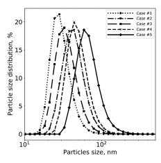
Figure 1. Mg(OH)<sub>2</sub> PSDs for Cases #1–5. PSDs were obtained after 5 min of ultrasound treatment and using PAA as a dispersant. Measurements were carried out using the Malvern Zetasizer Nano 7SD.
