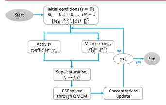
Figure 3. 1D model flow chart.
