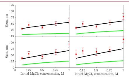
Figure 7. Characteristic sizes, from left to right and top to bottom,  $d_{10}$ ,  $d_{21}$ ,  $d_{32}$ ,  $d_{43}$ , derived from the measured PSD (red symbols) and predicted by the model (black lines—all phenomena, green line—molecular processes only), versus the initial MgCl<sub>2</sub> concentrations.
