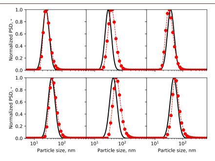
**Figure 9.** Reconstructed PSDs from their moments, compared with the experimental ones. Each comparison refers to the concentration set investigated #1, #2, #3, #4, #5, and #6. Black lines are the PSDs from simulations, whereas the red dotted lines are the PSDs from experimental tests (#1, top-left/#2, top-middle/#3, top-right/#4, bottom-left/#5, bottom-middle/#6, bottom-right).
