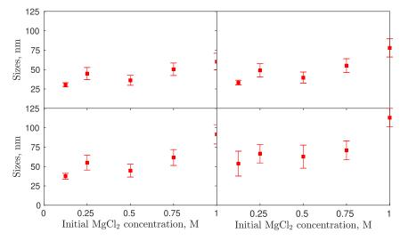
Figure 2. Characteristic sizes from left to right and top to bottom,  $d_{10}$ ,  $d_{21}$ ,  $d_{32}$ ,  $d_{43}$ , derived from PSDs, versus initial MgCl<sub>2</sub> concentrations ( $d_{10}$ , top-left/d top-right/ $d_{32}$  bottom-left/ $d_{43}$  bottom-right).
